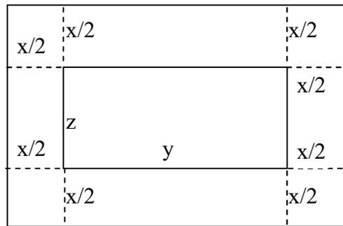
$$\text{also: } A(x,y,z) = 2(x+z) * (x+y) \quad (= 2x^2 + 2xz + 2xy + 2zy)$$
